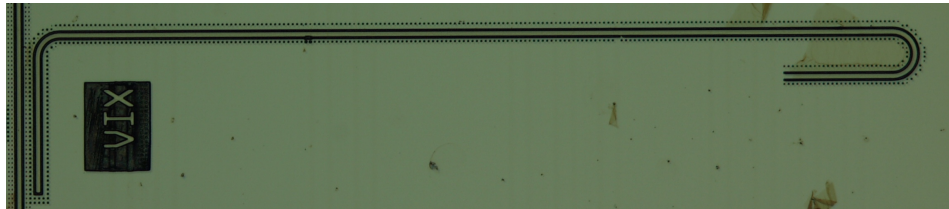
Fig. 1.4: \frac{\lambda}{4} -resonator coupled inductively to a feedline. The brighter regions are superconductor; the small dots in the ground plane are flux traps. The resonator was fabricated during this work.
